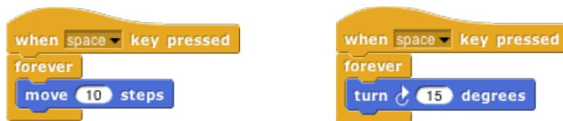
When you press the space key, the sprite should turn forever in a circle, because the **move** and **turn** blocks are run in parallel. (To stop the program, click the red stop sign at the right end of the tool bar.)
